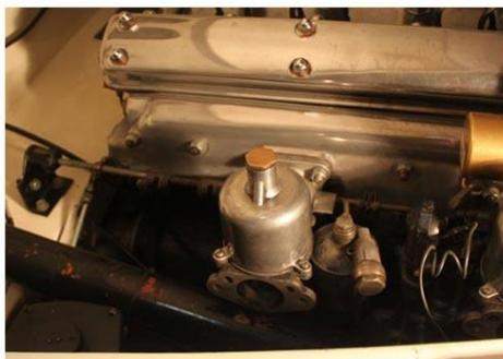
One of the most effective ways to give an engine more power is to get more air and fuel into it. Fitting larger carburettors or more of them is the easiest way to do this. SU carburettors were fitted to all XKs with twins on all but late 150 S models, which had three, as on the E-type. There are several possible conversions to larger carburettors or triple fitments and the ultimate is to fit triple twin choke Webers if you like power and pumping gas.
