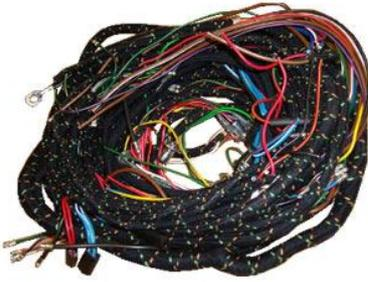
The wiring on XKs is hidden away and old wiring poses both a fire and reliability hazard. Rewiring is often the answer and for this our replacement loom is a must. As to upgrading, then replacing dynamos with alternators or fitting high power lightweight starters are two popular mods. Converting from positive to negative earth is also something that can be necessary in some cases.
