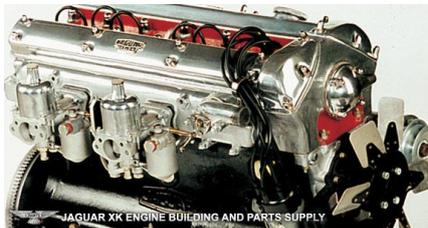
Like the heads, various blocks were used on XKs and of course capacity went from 3.4 to 3.8 and later in the E-type to 4.2 litre. Knowing the differences is important if you are changing engines.
