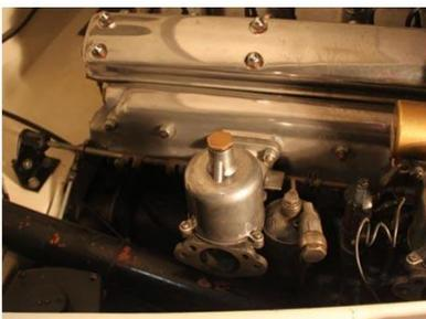
Unless you have them, going from two 1¾ in to two 2 in SUs, with the enlargement of the inlet manifold ports, is the first step. This is relatively easy and cost effective. However remember that any tuning will increase the stresses in the engine so be cautious if your engine is a bit tired.
