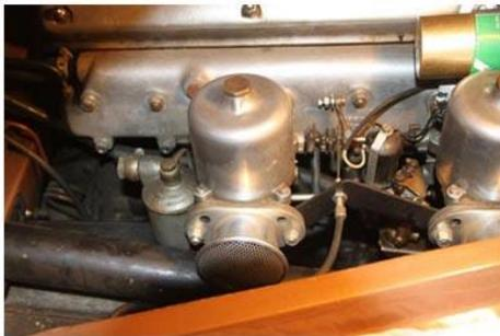
Going to three SUs and in particular three Webers is going to increase the fuel consumption and that means the fuel pump working harder. Fitting a high pressure pump is the answer. Lastly, tempting as it is to have bell mouth intakes sticking out of your carburetors, if that is your choice, at least fit ones with metal gauze over them to reduce the rubbish that gets sucked into the engine.
