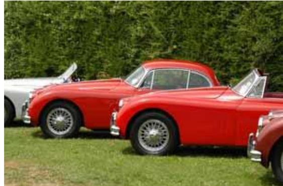
There are three wire wheels available that closely replicate the original 16" wheels fitted to XKs. Two have 60 spokes – one having a 5" wide rim and the other 6". There are no 5 ½" wide 16" wheels available. There is also a 6" option in the same style but with 72 spokes for extra strength. The 5" wheel can take 185 R16 tyres and the others either 185 x 16 or 215/65R16. Current wheels take tubeless tyres but if you have older ones you may need tubes.
