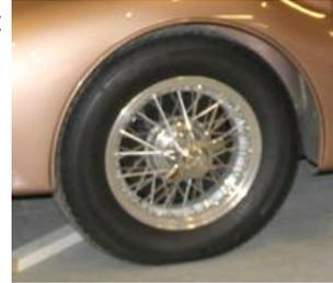
If you have front wheel shake at low speeds then of course the first job is to check the wheels are balanced OK. If you have wire wheels make sure you get them balanced by someone with the right equipment. Kwik Fits and the like generally don't have the dummy hubs to mount the splined centres on wire wheels so make sure the balancing is done correctly. This will also check that the wheels and tyres are running true - another cause of wobble.
