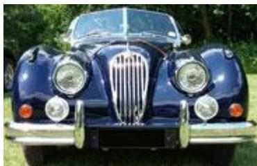
Jaguar XK140's have a level of sophistication compared to the earlier XK120. Re-designed to include rack and pinion steering, telescopic shock absorber damping to the rear, an overdrive gearbox option along with a more powerful engine and updated to 2 inch carburettors.
