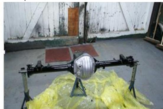
The Salisbury HA4 axle continued through the production of the 150. A 3.54:1 ratio axle was fitted to all 3.4 litre cars and 3.8 models built for the USA, Canada and Mexico, with overdrive models for those markets having a 4.09:1 axle. For other
