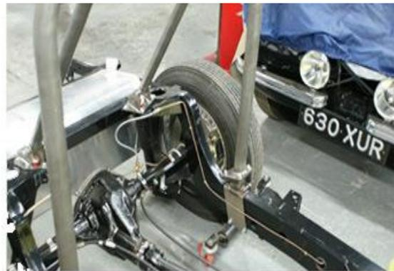
For 140s the story is far clearer. Only Salisbury 4HA axles were used with a standard ratio of 3.54:1 and options of 3.31:1 and 4.27:1. Overdrive models used 4.09:1. The half shafts and hubs for both five stud and splined wheels were the same as on 120s with Salisbury axles. There were a few small mechanical differences introduced, relating to the lock tabs and differential (diff) bolts, but that was it.
